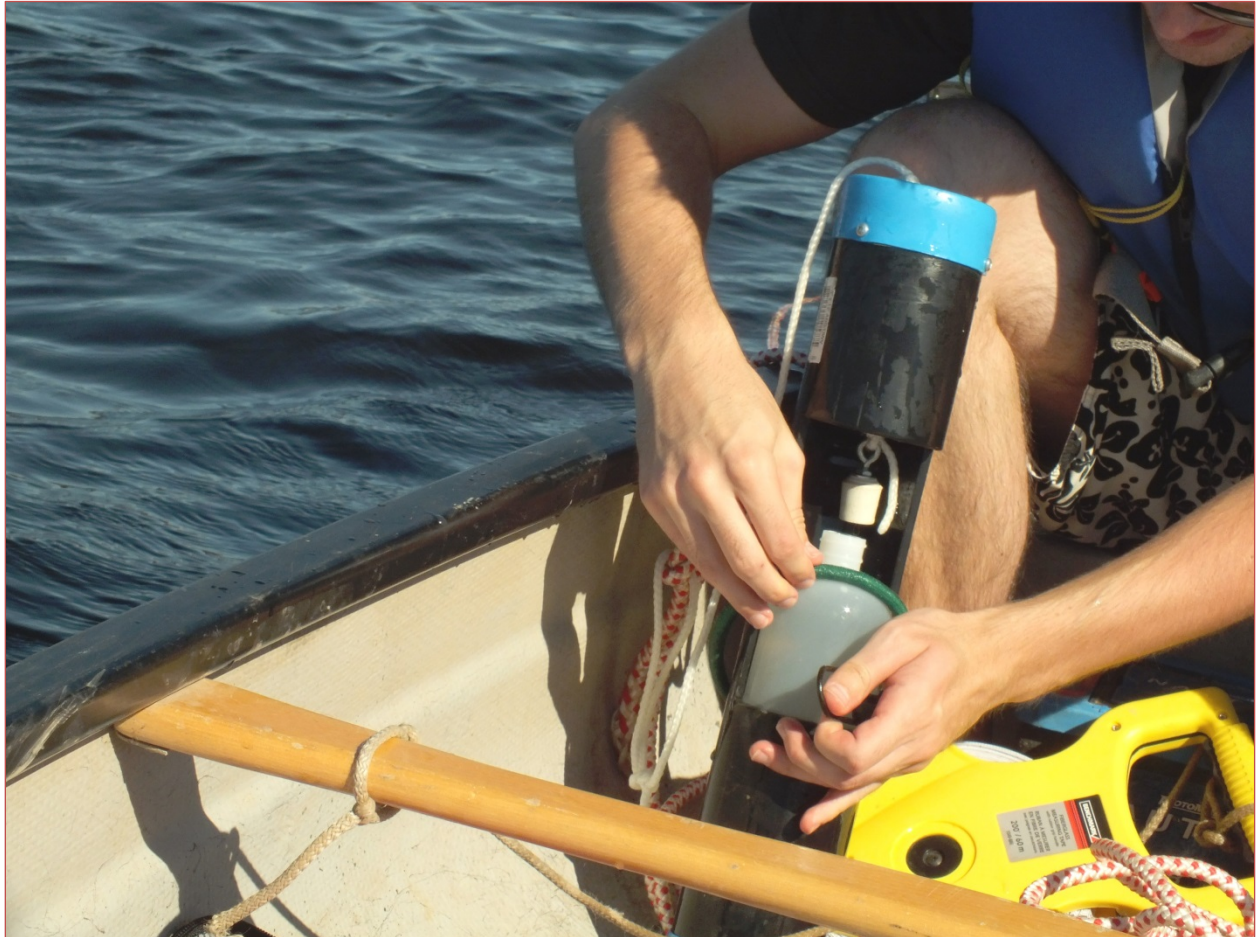
FIGURE 2-2 SAMPLING DEVICE USED TO COLLECT WATER SAMPLES FROM MONITORED LAKES
